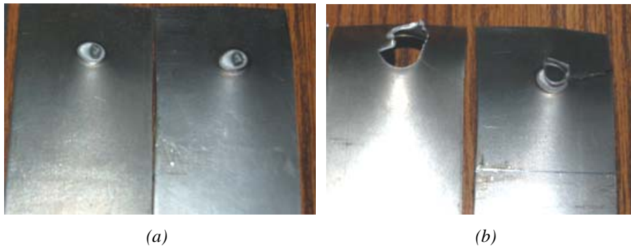
Figure 5 Failure modes of spot welds during tensile-shear test a) interfacial and b) pullout failure mode
